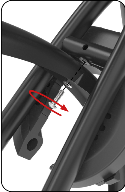
9A - Rear fender with a slotted hole
