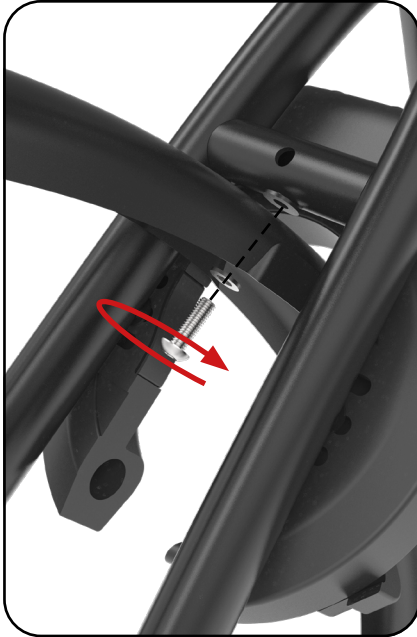
5A - Rear fender with a slotted hole
