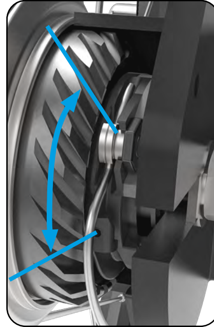
15 - Fitting the shifting cable
