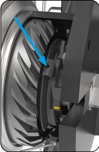
14 - Preparing the cassette joint for fitting the shifting cable
